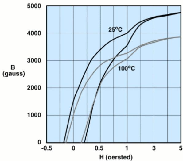
Measured on an 18/10/6mm toroid at 10kHz.
