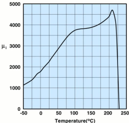
Measured on an 18/10/6mm toroid at 100kHz.
