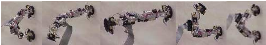
Fig.11. Micro-robot climbing the wall
