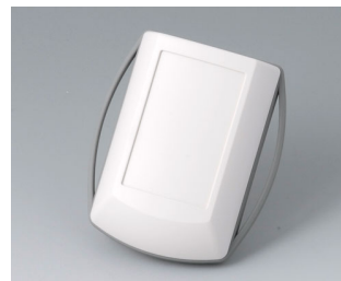
B7040227 ERGO-CASE XS ABS (UL 94 HB) off-white RAL 9002 3.23"x2.20"x0.94" IP 42
