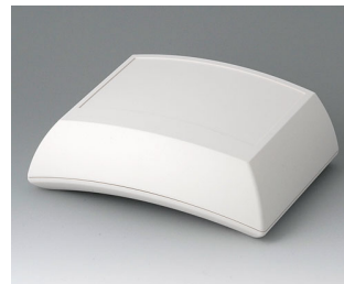
B7025207 ERGO-CASE L, high ABS (UL 94 HB) off-white RAL 9002 5.91"x7.87"x2.72" IP 54 opt.
