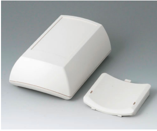
B7015107 ERGO-CASE M, high ABS (UL 94 HB) off-white RAL 9002 5.91"x3.94"x2.17" IP 54 opt.
