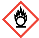
Flame over Circle Oxidizers
