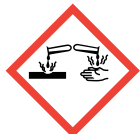
Corrosion Skin Corrosion/Burns and Eye Damage
