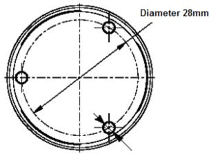
PCB with holes to heat stake the holder
