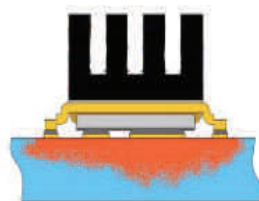
⑦ Mounted to a PCB with small clip heatsink (still air)
