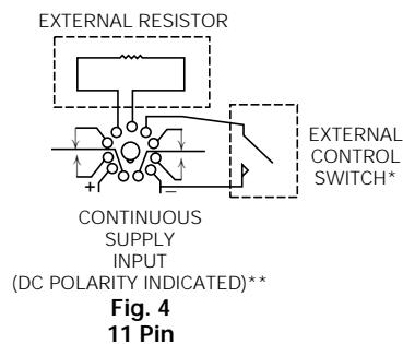
\* If control switch is closed when power is applied, relay will immediately energize. A 50 millisecond minimum switch closure is required. IMPORTANT: A dry circuit switch is recommended. A "dry circuit" switch is one rated to reliably switch currents of less than 50mA. Use of a switch rated for other than dry circuit may result in failure of the time delay relay to function properly.
