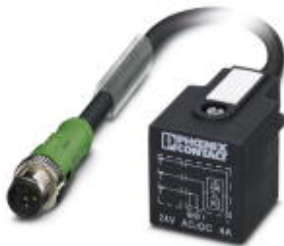
Sensor/Actuator cable, PUR halogen-free, Black-gray RAL 7021, Plug straight M12, A-coded, on Valve connector A, with 1 LED, connected with Z diode, Cable length: 0.3 m
