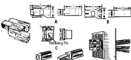
The connector modules have dovetail locking grooves molded into the housing. The housing can be assembled to form a multi-pole connector.
