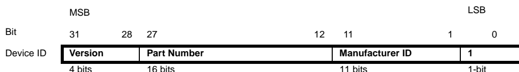
Figure 26-1. The Format of the Device Identification Register
