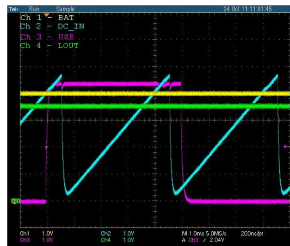
Figure 7. TPS22933A with Varying Inputs and Stable LOUT
