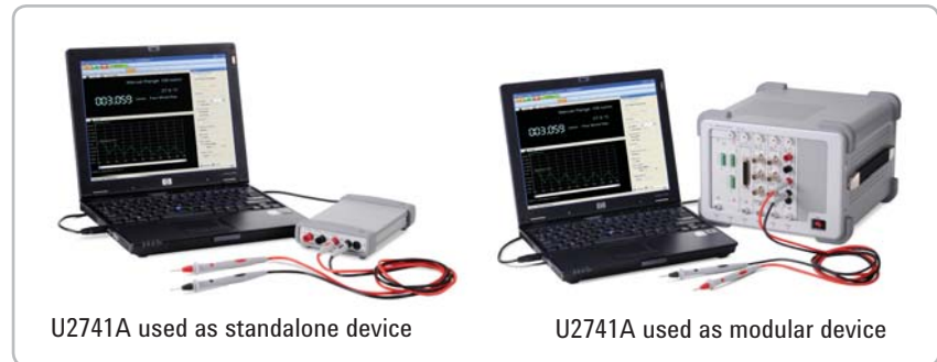
Figure 1. The U2741A DMM showing dual-play capability
