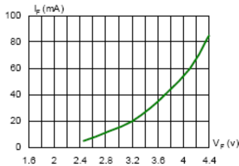
Fig.1 Forward Current vs. Forward Voltage
