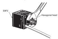
• When attaching the Mounting Bracket to the Sensor, make sure that each M3 screw is tightened to a torque of 0.5 N·m max.
