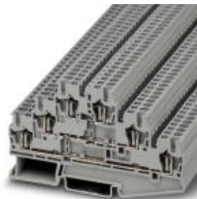
Multi-level terminal block, with diode1N4007, Connection method: Spring-cage connection, Cross section: 0.08 mm<sup>2</sup> - 4 mm<sup>2</sup>, AWG: 28 - 12, Width: 5.2 mm, Color: gray, Mounting type: NS 35/7,5, NS 35/15
