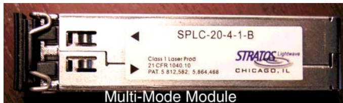
Figure 13-2 Multi-Mode SFP Module — Stratos Part# SPLC-20-4-1-B — Harris Part # GBE-OPT-MM
