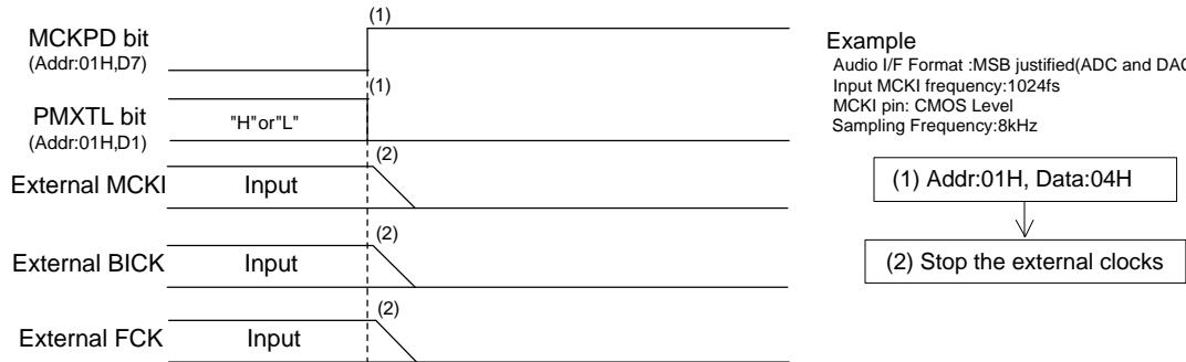
Figure 43. Stop of Clock Sequence (4)
