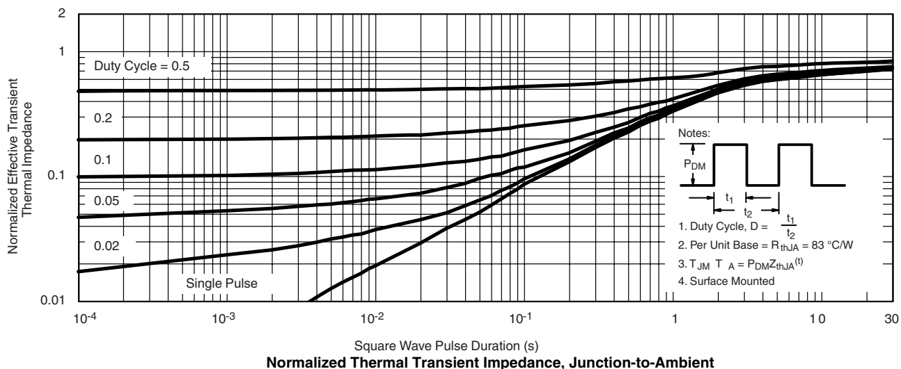
Normalized Thermal Transient Impedance, Junction-to-Ambient
