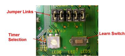
The jumper links configure the outputs to be Momentary, Latching or Timed.
