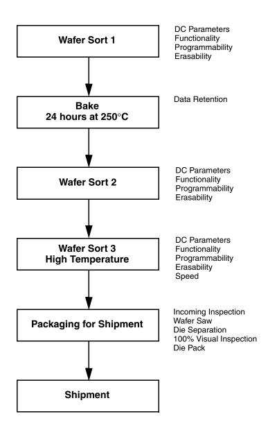
Figure 1. AMD KGD Product Test Flow
