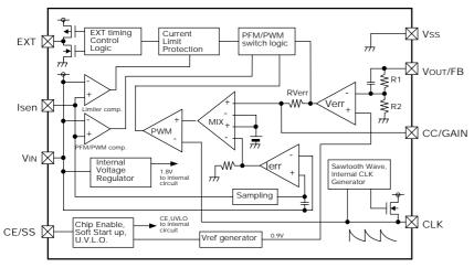
The output of EXT pin is switched "H" and "L" between XC9101/02 series and XC9201/02 series.
