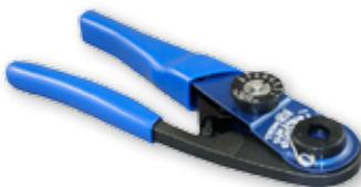
Standard M22520/2-01 crimper for use with standard size #23 Mighty Mouse contacts. Crimp tools perform precision eight indent crimps for gas-tight wire terminations and excellent tensile strength. Adjustment wheel has 8 settings. Ratchet mechanism prevents improper crimps. Use with bayonet-type positioners. Check calibration with M22520/3 gages. Length is 6.75 inches, weight is approx. 10 oz.
