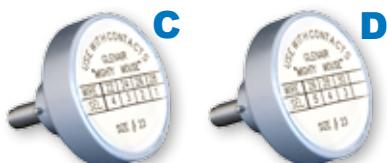
These bayonet-type positioners hold contacts at correct height for crimping with M22520/2 type miniature step adjustable tools, above. Face plate shows correct tool settings. "C" Positioner is for standard size #23 contacts. #22-#28 AWG. Use with 809-015 crimp tool. "D" Positioner is for small bore size #23 contacts. #26-#30 AWG. Use with 809-015 crimp tool.
