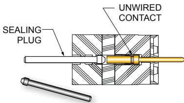
Grommet sealing plugs are used to seal unwired contact cavities. The size #23 sealing plug is specially designed to fit Glenair Series 80 grommets. After installing unwired contacts into unused cavities, insert knob end of sealing plug into grommet until it bottoms against the unwired contact per illustration. Install sealing plugs with standard contact insertion/extraction tools. The size #23 plug is polyphenylsulphone.
