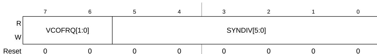
Figure 8-3. S12XECRG Synthesizer Register (SYNR)
