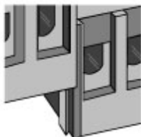
Dovetail Interlocking Feature
