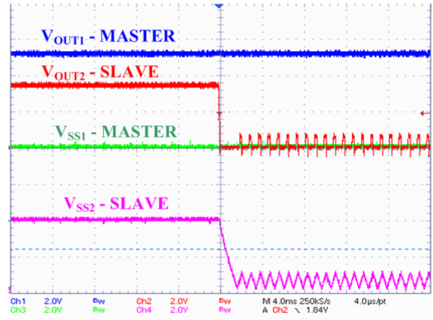
Figure 64. Master Voltage – End of Augmented OLM
