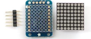
When you buy a pack from Adafruit, it comes with the fully tested and assembled backpack as well as a 8x8 matrix in one of the colors we provide (say, red, yellow or green). You'll need to solder the matrix onto the backpack but its an easy task.
