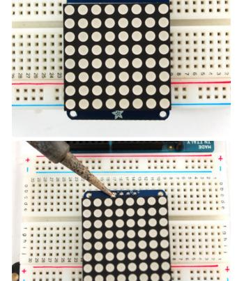
Place the soldered backpack on top of the header.
