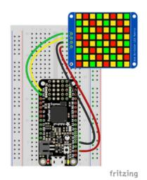
Microcontroller 3V to LED Matrix VIN
