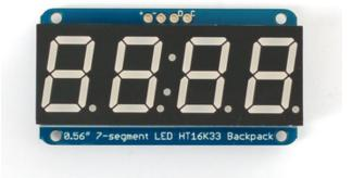
Remove the parts from packaging and place the LED matrix OVER the silkscreen side. DO NOT PUT THE DISPLAY ON UPSIDE DOWN OR IT WONT WORK!! Check the image below to make sure the 'decimal point' dots are on the bottom, matching the silkscreen.
