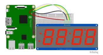
Raspberry Pi 3.3V to 7-Segment Display IO
