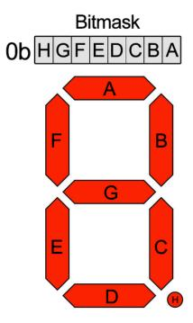
The bitmask is a single 8-bit number that can be passed in as a single Hexadecimal, Decimal, or binary number. This will use a couple different methods to display 8.8.EE:
