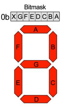
The bitmask is a single 8-bit number that can be passed in as a single Hexidecimal, Decimal, or binary number. This will use a couple different methods to display 8E8E:
