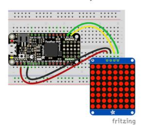
Microcontroller 3V to LED Matrix VIN
