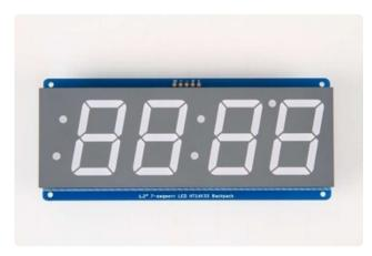
Remove the parts from packaging and place the LED matrix OVER the silkscreen side. DO NOT PUT THE DISPLAY ON UPSIDE DOWN OR IT WONT WORK!!
