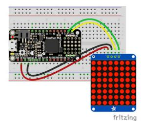
Microcontroller 3V to LED Matrix VIN
