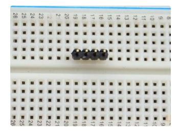
Break off a piece of male header, 4 pins long. Plug the **long ends** into a solderless breadboard.
