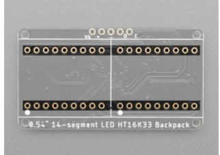
These two rows of through-hole pads are for soldering the alphanumeric LED displays onto the backpack. See the <a href="#">Assembly page</a> (https://adafru.it/11dU) for details on attaching the displays properly.
