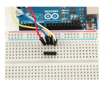
Now you're ready to wire it up to a microcontroller. We'll assume you want to use a 4pin header. You can also of course solder wires directly. Place a 4-pin piece of header with the LONG pins down into the breadboard.
