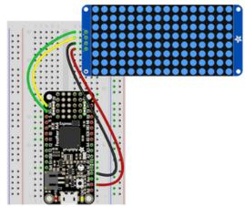
Microcontroller 3V to LED Matrix VIN
