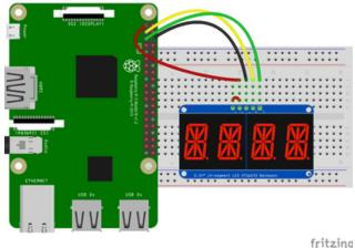
Raspberry Pi 3.3V to AlphaNumeric Display I2C VIN
