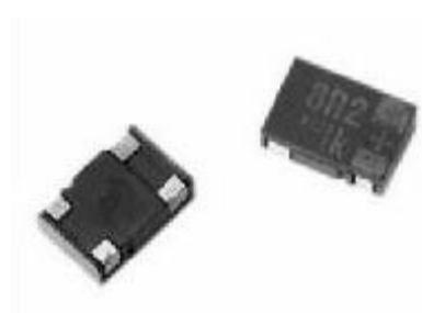
Type ESR SMT capacitors are polarized, aluminum capacitors which use a highly conductive solid polymer as the electrolyte.
