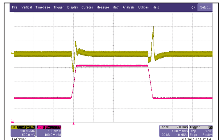
Figure 6: Output voltage response to step-change in input voltage (180V - 425V - 180V), at 12.5A load current. Load cap: 15μF tantalum capacitor and 1uF ceramic cap. Ch 1: V out (500mV/div), Ch 2: V in (100V/div).
