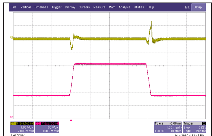
Figure 6: Output voltage response to step-change in input voltage (180V - 425V - 180V), at 6.25A load current. Load cap: 15μF tantalum capacitor and 1uF ceramic cap. Ch 1: V out (1V/div), Ch 2: V in (100V/div).
