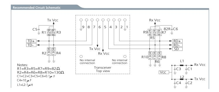
The split-load terminations for ECL signals need to be located at the input of devices receiving those ECL signals. The power supply filtering is required for good EMI performance. Use short tracks from the inductor L1/L2 to the module Rx  $V_{cc}$  and Tx  $V_{cc}$ . A GND plane under the module is required for good EMI and sensitivity performance.
