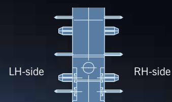
Side definition with terminals and location pins
