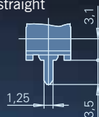
PCB terminal 1,3x0,5 mm straight
