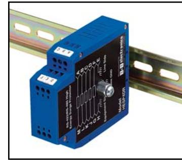
Model HESP4DR is designed to help protect against lightning strikes, power surges, and other types of voltage disturbances to components on a DIN rail. Five RS-422/485 signals on terminal blocks are supported with a clamping voltage of approximately 6.8 volts. The HESP4DR offers three stages of protection starting with a gas discharge tube followed by a series resistor and finally a Transient Voltage Suppressor (TVS).
