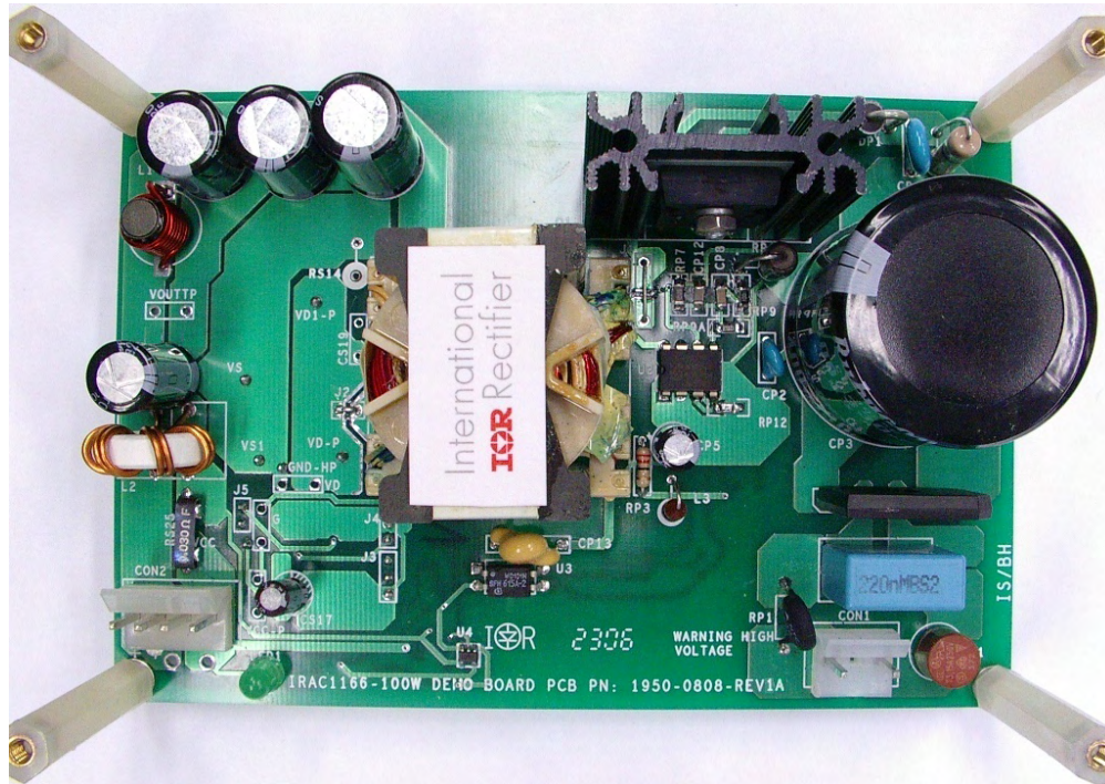
Figure 2A. Top side of the IRAC1166-100W Demo Board
