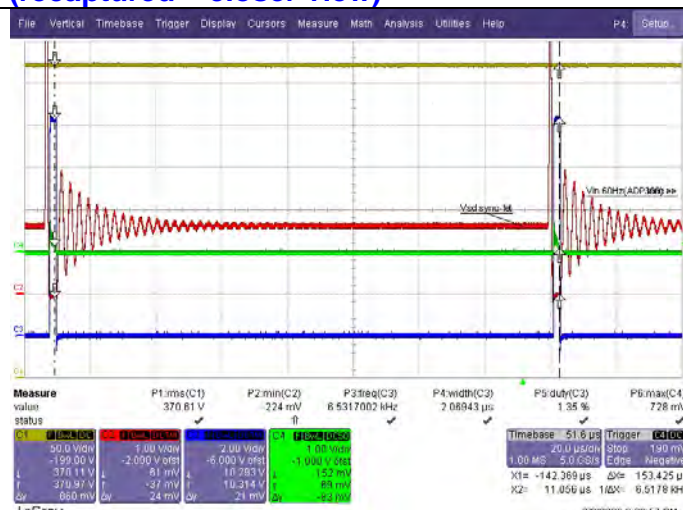
Fig. 6H - 265Vac in, 16Vout / no load (recaptured – closer view)
