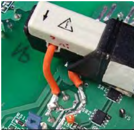
Fig. 4B Recommended probing of secondary current waveform.
