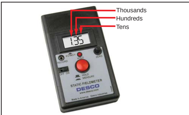
Figure 2. Reading the Digital Static Field Meter
