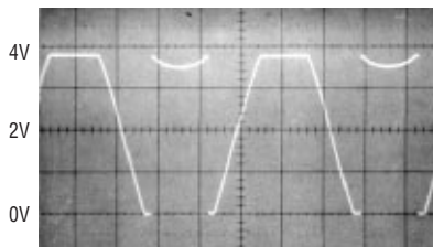
LM324, LM358, OP-20 EXHIBIT OUTPUT PHASE REVERSAL
