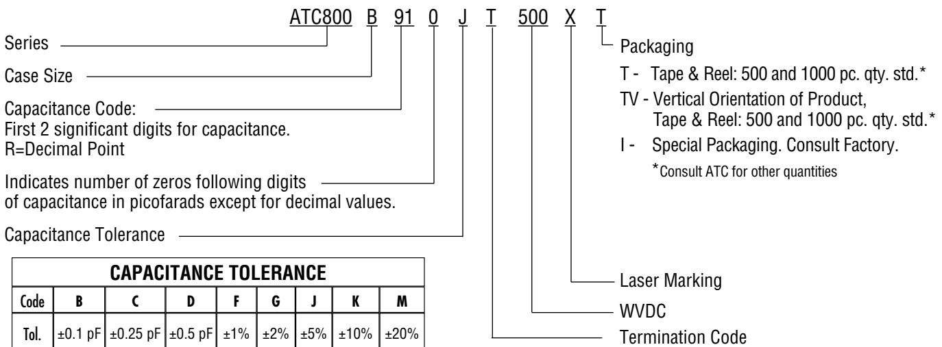
The above part number refers to a 800 B Series (case size B) 91 pF capacitor, J tolerance (±5%), 500 WVDC, with T termination (Tin Plated over Nickel Barrier Termination, RoHS Compliant), laser marking and tape and reel packaging.
