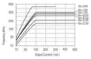
Switching Frequency Vs Load (Vin=30~72V)
