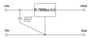
The converter has a built in soft start circuit. Rapidly changing the input voltage from  $Vin(min) \leftrightarrow Vin(max)$  can bypass this circuit and damage the converter.
