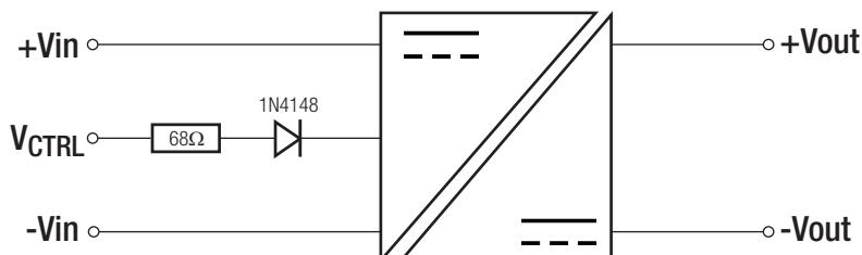
DC-DC ON: Open or  $0\text{V} < V_r < 0.8\text{VDC}$
