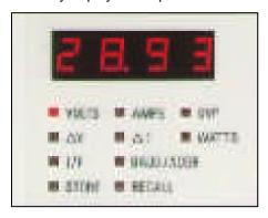
All key board en tries ap pear on this display for inspection before they are actioned by press ing the "con firm" key.
