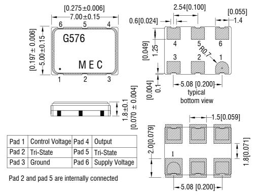
Rounded pad is pad No. 1. Count counter-clockwise when looking at top view. Count clockwise when looking at bottom view.
