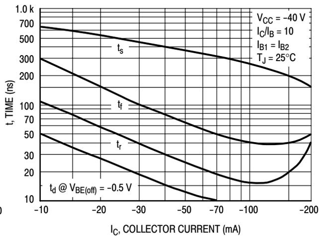
**Figure 8. Switching Times**
