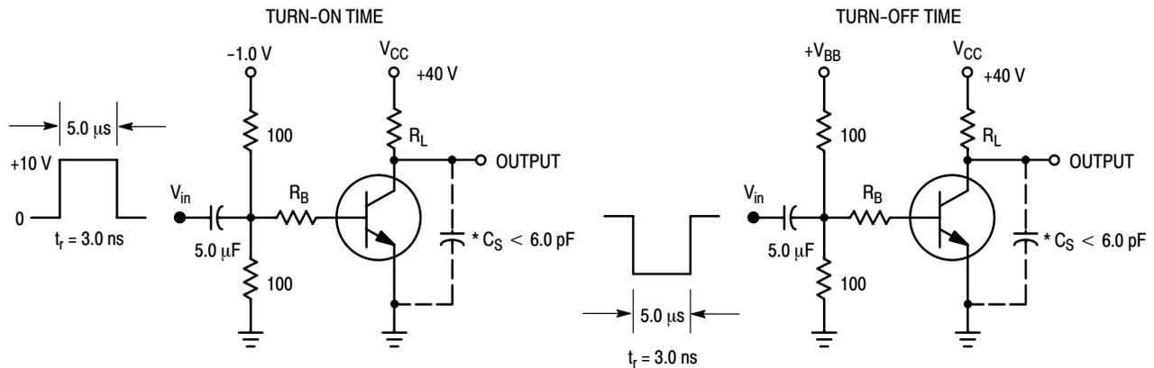
\*Total Shunt Capacitance of Test Jig and Connectors For PNP Test Circuits, Reverse All Voltage Polarities
