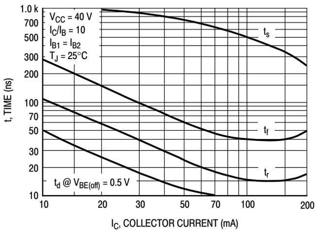
**Figure 7. Switching Times**
