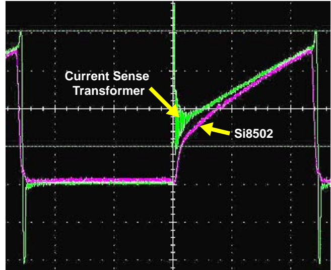
Figure 8. Leading-Edge Noise Suppression Waveforms (200 kHz, 9.3 A Load)
