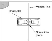
Screw each wall clip into place using a cross head screwdriver. Ensure they are central to the line and horizontal in orientation as shown.
