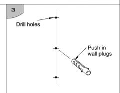
Where marked, drill a hole for each wall clip using a 6mm drill bit to a depth of 35mm. Insert a wall plug into each hole so that they are flush with the wall surface.
