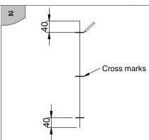
Mark across the line where you want to position the wall clips. There should be a wall clip 40mm from each end with the others equally spaced between them.
