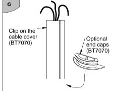
Finally push on the cable cover so that it clips into place. If cables enter or exit through a hole in the wall, you may push-in one or both of the plastic end caps.
