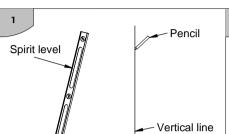
Draw a pencil line on the wall where you wish the centre of the cable manager to be. Use a long spirit level to ensure this line is vertical.
