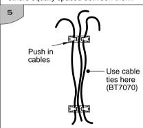
Push cables through the gap in the front of the wall clips so they are retained. Use the cable ties to help group the cables at points inbetween the wall clips. Trim off excess.
