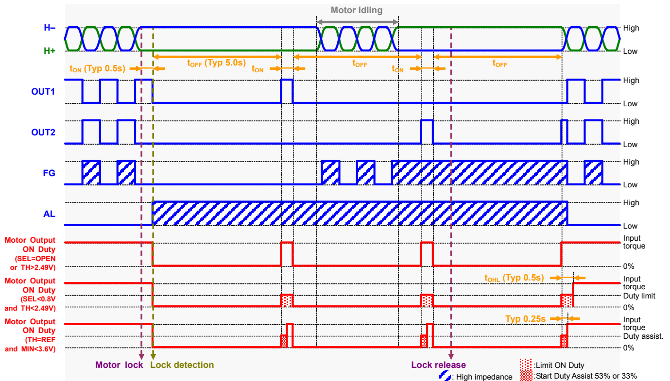
Figure 63. Lock Protection (Incorporated Counter System) Timing Chart
