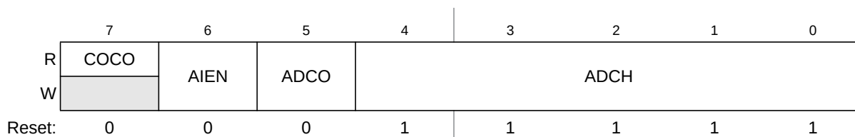
Figure 10-3. Status and Control Register (ADCSC1)
