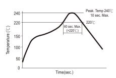
Remark : The curve applies only to the "Hot Air Reflow Soldering"
