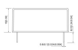
Case No.IRM02 Unit:mm[inch] Tolerance:±0.5[±0.02] unless otherwise specified
