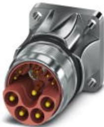
Device connector for front wall, straight, shielded: Yes, Screw locking, M23, No. of pos.: 4+4+4+PE / 3+N+PE, type of contact: Pin, Crimp connection, Axial O-ring, 4x Ø 3.2, flange dimensions: 26 mm x 26 mm
