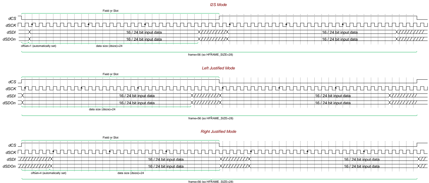
Figure 6-1: Data Interface Timing Diagram I2S/LJ/RJ
