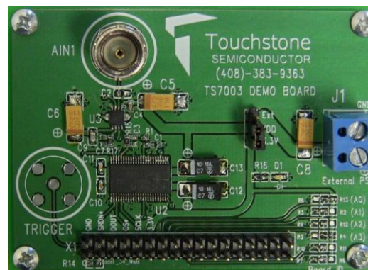
Figure 2. TS7003 Evaluation Board
