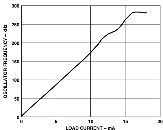
TPC 12. Oscillator Frequency vs. Load Current
