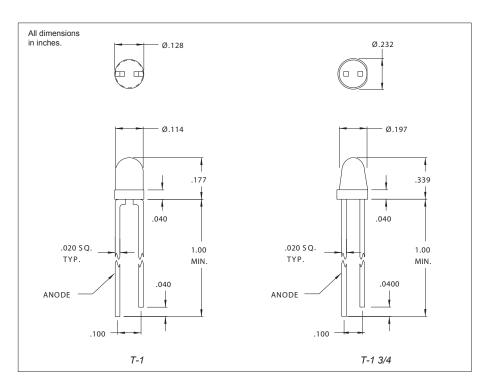
These revolutionary new LED lamps emit a true blue color (430 nm) for those design engineers looking for that fourth status color. Lamps are manufactured with state of the art Silicon Carbide (SIC) technology.
